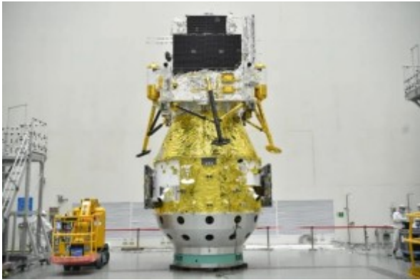
The Chang'e-6 spacecraft stack shows a lunar rover attached to the mission lander. Credit: CAST
