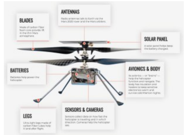
A graphic show the parts of the Ingenuity helicopter.
