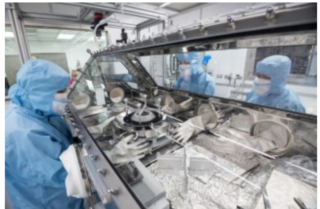
OSIRIS-REx astromaterials processors, from left, Rachel Funk, Julia Plummer, and Jannatul Ferdous, prepare to lift the top plate of the Touch-and-Go Sample Acquisition Mechanism (TAGSAM) head and pour the final portion of asteroid rocks and dust into sample trays below. Credit: NASA/Robert Markowitz
