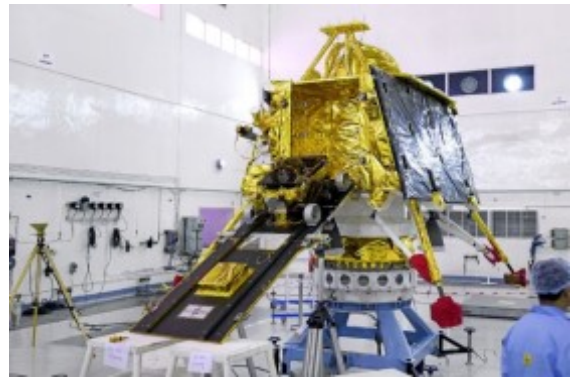
The Vikram lander with its ramp deployed to show how the rover will roll onto the surface. Credit: ISRO
