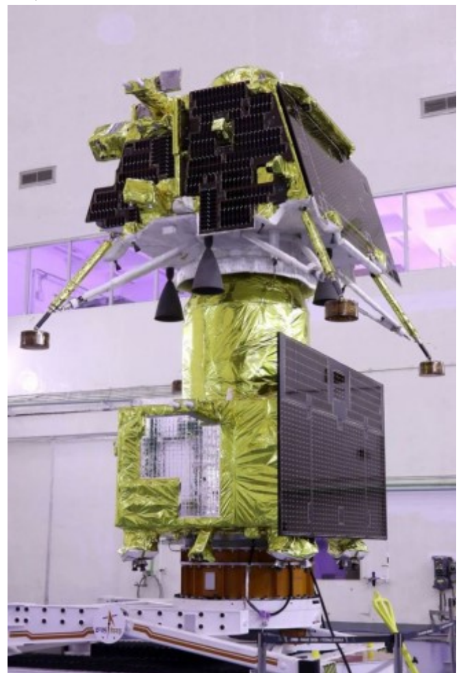
The Chandrayaan-3 Integrated Module with the Vikram lander plus Pragyan rover (top) and the Propulsion Module (bottom). (Credit: Indian Space Resource Organization)
