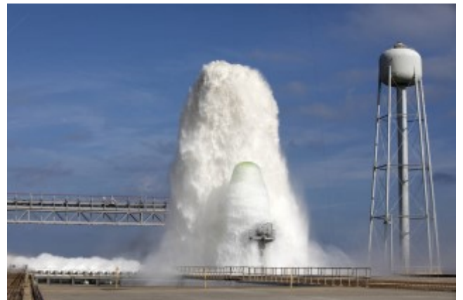
The IOP/SS system deploys almost a half-million gallons of water in one minute to protect the SLS during launch. Credit: NASA
