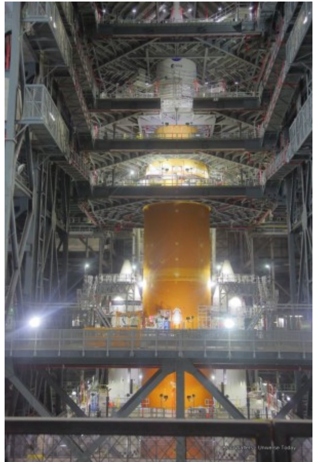
The stack of the Space Launch System rocket in the Vehicle Assembly Building at Kennedy Space Center earlier this year. Credit and copyright: Alan Walters, for Universe Today.
