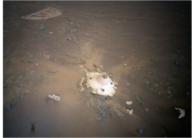
This image of the Perseverance rover's parachute and backshell was taken by the Ingenuity helicopter during its 26th flight on April 22, 2022. Credit: NASA/JPL-Caltech
