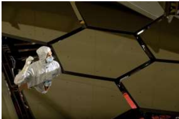
A primary mirror segment of the James Webb Space Telescope, made of beryllium. Credit: NASA/MSFC/David Higginbotham/Emmett Given
