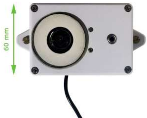
Example of a standardized TESS photometer. Credit: TESS / Stars4all
