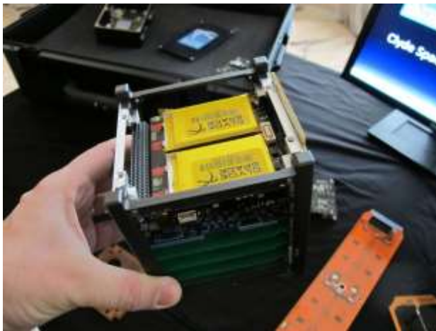
Example of a 1U CubeSat. Credit: Wikipedia user Svobodat
