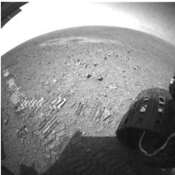
This image shows a close-up of track marks left by the Curiosity rover. Holes in the rover's wheels, seen here in this view, leave imprints in the tracks that can be used to help the rover drive more accurately. The imprint is Morse code for 'JPL,' and aids in tracking how far the rover has traveled. Credit: NASA/JPL-Caltech.
