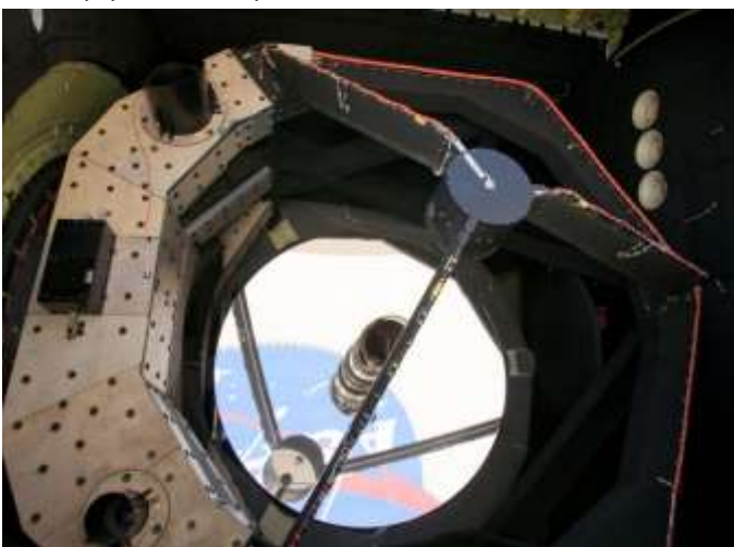
A close-up of SOFIA's telescope and primary mirror. Credit: NASA/Tom Tschida
