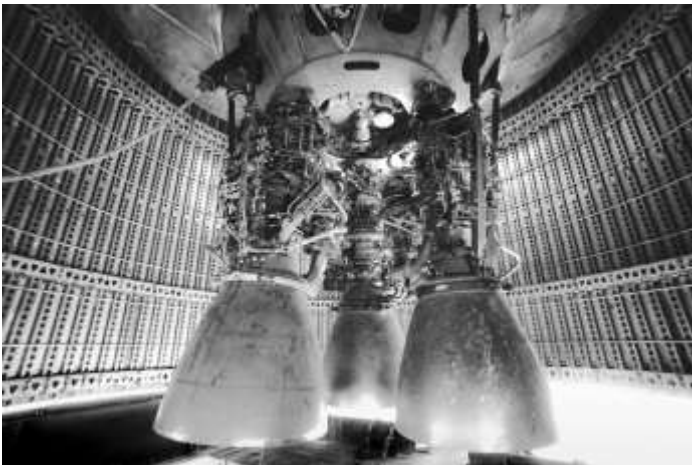
The Mk.1’s interior, showing its three Raptor engines. Credit: SpaceX
