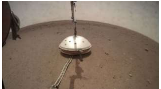
The InSight Lander’s seismometer underneath its protective wind and thermal shield. Image Credit: NASA/JPL-Caltech
