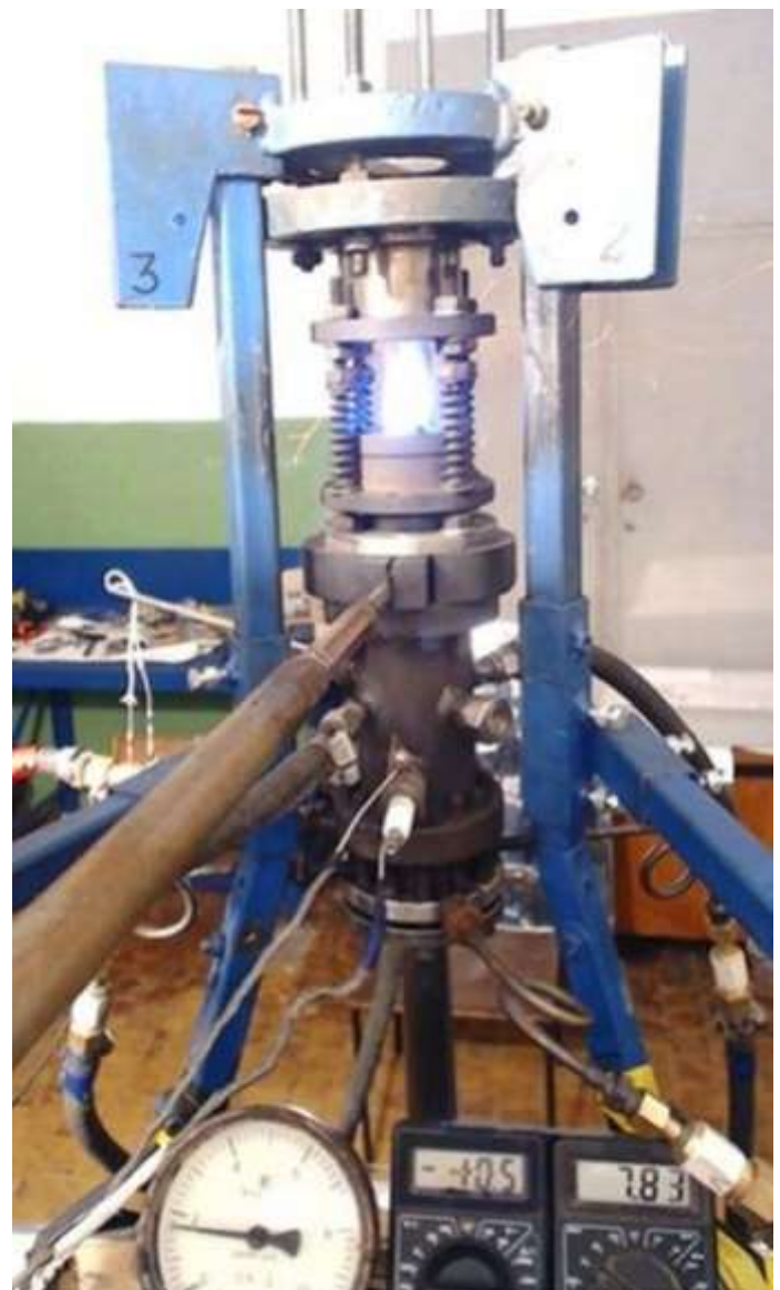
The autophage engine, being tested at the Dnipro testing lab in the Ukraine. Credit: University of Glasgow
