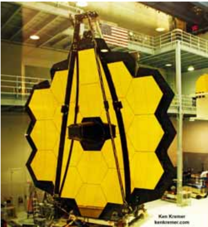
The 18-segment gold coated primary mirror of NASA’s James Webb Space Telescope is raised into vertical alignment in the largest clean room at the agency’s Goddard Space Flight Center in Greenbelt, Maryland, on Nov. 2, 2016. The secondary mirror mount booms are folded down into stowed for launch configuration. Credit: Ken Kremer/kenkremer.com
