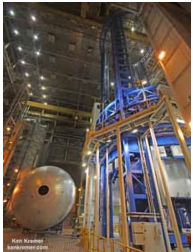
The newly assembled first liquid hydrogen tank, also called the qualification test article, for NASA’s new Space Launch System (SLS) heavy lift rocket lies horizontally beside the Vertical Assembly Center robotic weld machine (blue) on July 22, 2016. It was lifted out of the welder (top) after final welding was just completed at NASA’s Michoud Assembly Facility in New Orleans. Credit: Ken Kremer/kenkremer.com
