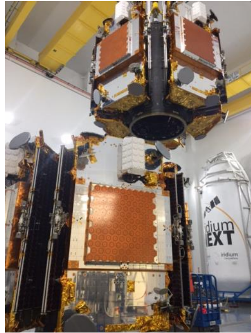
IridiumNEXT satellites being fueled, pressurized & stacked on dispenser tiers at Vandenberg AFB for Falcon 9 launch. Credit: Iridium
