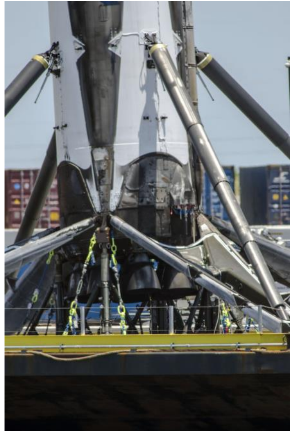
A close-up of restraints installed at the base of the Falcon 9 booster for stabilization as the rocket returned to Port Canaveral on Thursday. Credit: James Murati/Bionetics
