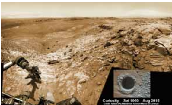
Curiosity extends robotic arm and conducts sample drilling at "Buckskin" rock target at bright toned "Lion" outcrop at the base of Mount Sharp on Mars, seen at right. Gale Crater eroded rim seen in the distant background at left, in this composite multisol mosaic of navcam raw images taken to Sol 1059, July 30, 2015. Navcam camera raw images stitched and colorized. Inset: MAHLI color camera up close image of full depth drill hole at "Buckskin" rock target on Sol 1060. Credit: NASA/JPL-Caltech/MSSS/Ken Kremer/kenkremer.com/Marco Di Lorenzo
