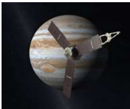
NASA's Juno spacecraft is powered by very large solar arrays. It began orbiting Jupiter in 2016. Credit: NASA/JPL-Caltech
