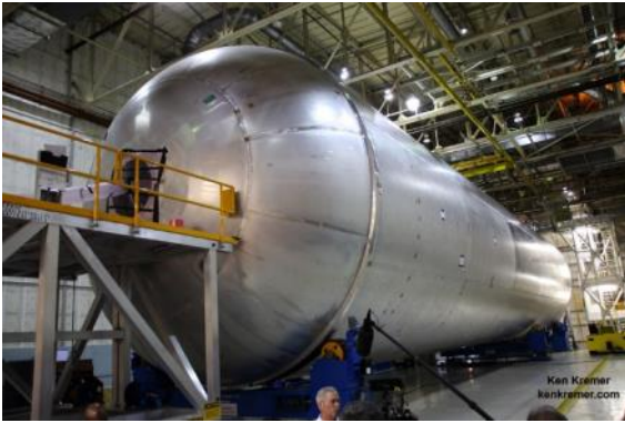
The liquid hydrogen tank qualification test article for NASA's new Space Launch System (SLS) heavy lift rocket lies horizontally after final welding was completed at NASA's Michoud Assembly Facility in New Orleans in July 2016. Credit: Ken Kremer/kenkremer.com
