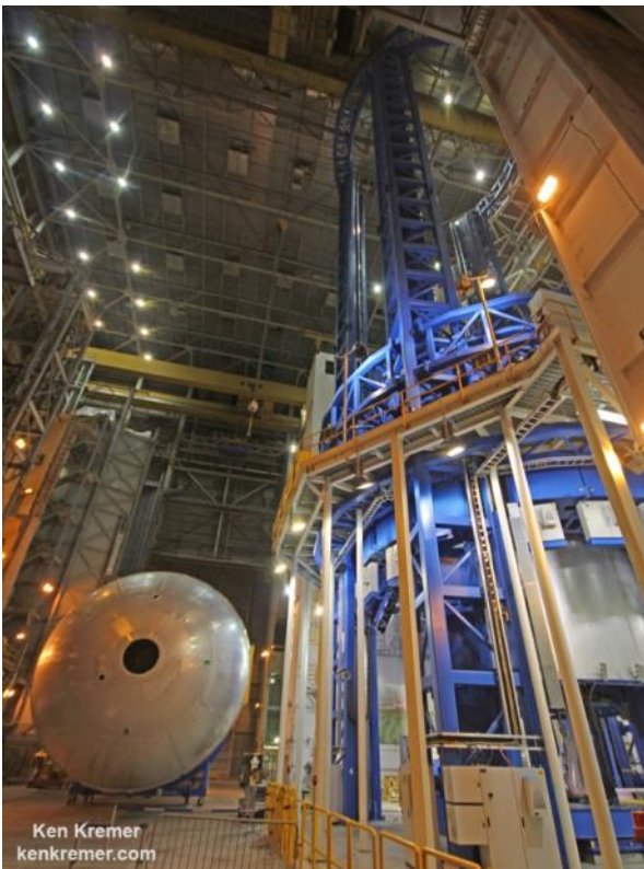
The newly assembled first liquid hydrogen tank, also called the qualification test article, for NASA's new Space Launch System (SLS) heavy lift rocket lies horizontally beside the Vertical Assembly Center robotic weld machine (blue) on July 22, 2016. It was lifted out of the welder (top) after final welding was just completed at NASA's Michoud Assembly Facility in New Orleans. Credit: Ken Kremer/kenkremer.com
