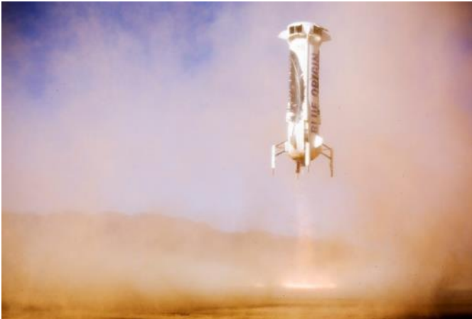
New Shepard comes in for a landing with drag brakes and landing gear deployed. Credit: Blue Origin.
