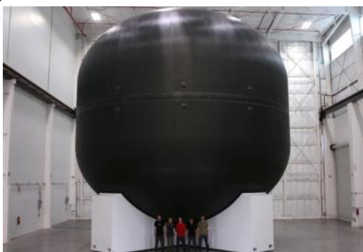
The ITS requires huge fuel tanks, one of which is seen here at SpaceX's production facility. Image: SpaceX
